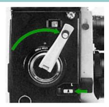
Open the back cover and make sure that a spool has been inserted into the take-up spool chamber.
